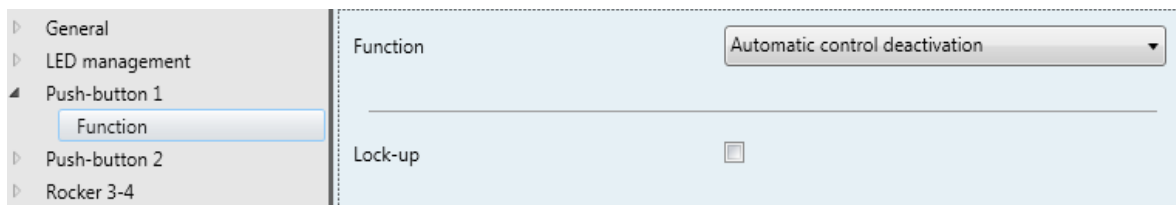
Figure 29: "Automatic control deactivation" parameter
