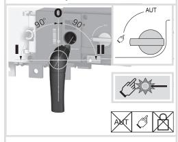
**7D. Padlocking mode (Standard: in position O)** Foreseen for max. 3 padlocks Ø 4-8mm
