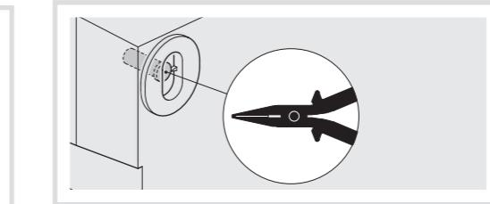
2. Locate the knob to indicate a precise value (30 °C for example) and remove it.
