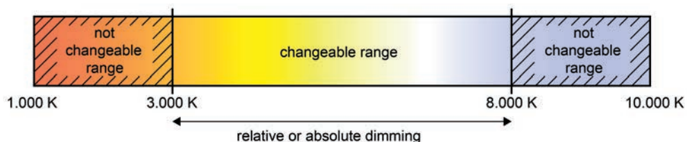
Figure 39: Automatic adjustment of the colour temperature to the set brightness Example with limited colour temperature range
