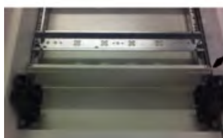
Direct screw connection on the mounting rails
