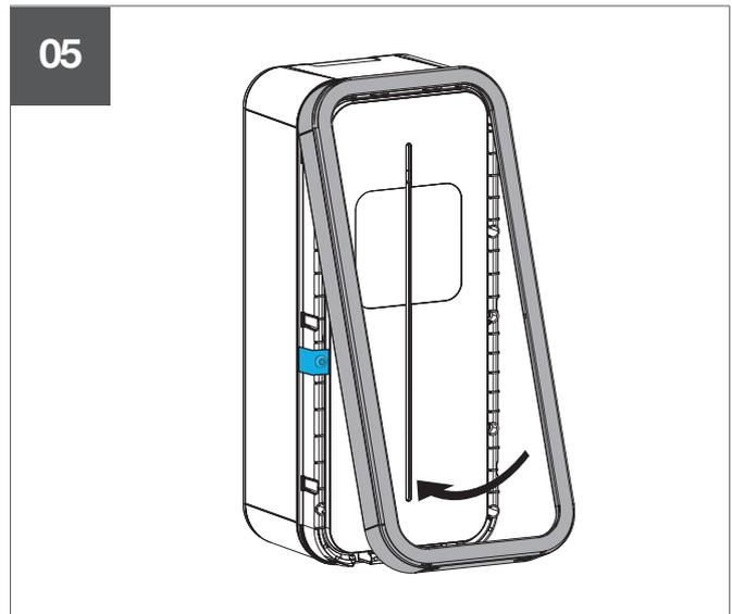
Fig 23: Kantenschutz anbringen
