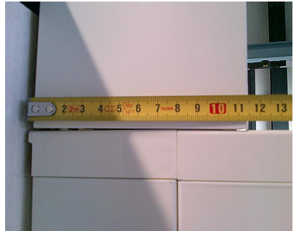
Cross section [mm] 115 x 155 or 155 x 115
