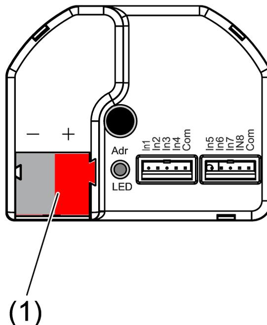
Figure 2: Raccord de bus
