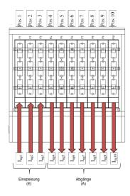
The ingoing current was evenly distributed over the supplying fuse rails:
