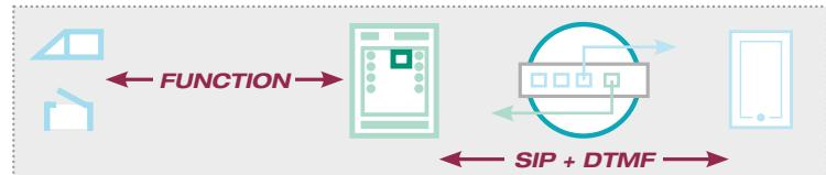
Thanks to the "Remote I/O" function, the SIP relay can be operated directly by the door module (via the outdoor caller unit). This means that it is possible to control electromechanical devices such as electrical latches or lighting in a secure manner.
