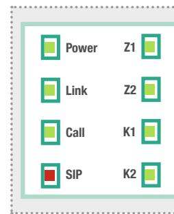
**Z1-Z2 (green)** Steady lighting: the contact is activated when a voltage ranging between 12 V and 24 V (VAC/VDC) is applied.
