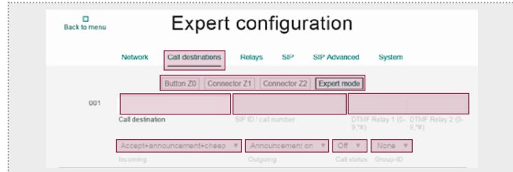
The behaviour of the Z0, Z1 or Z2 commands connected to the SIP relay is defined here. The “Expert mode” can be used to define a different command from the Z0, Z1 and Z2 commands.
