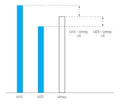
Voltage unbalance principle
