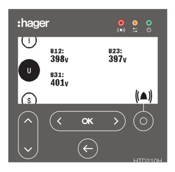
The notification windows for active alarms with a high priority level can be viewed after they have been cleared using the context-sensitive key when the Alarm icon is displayed.
