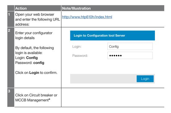
(\*) If you cannot click on Circuit breaker Management, check that the h3+ circuit breaker is correctly connected to the configuration tool. If the problem continues, refer to the user manual for the HTP610H configuration tool.
