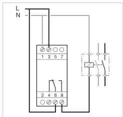
Image 2: EGN103 connection diagram (1 output)
