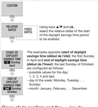
Press **ok** to confirm and the - key to return to the **Daylight Savings Time** menu.
