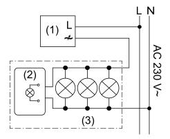
Figure 1: Example for connection in luminaire housing
