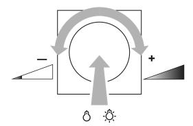
Figure 1: Switching light or adjusting brightness
