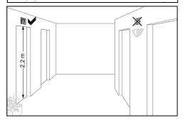
Fig. 4: Installation location of the motion detectors
