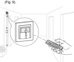
Fig. 9: Using the IR remote control
