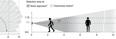
Fig. 6: Detection area of the motion detector for installation height 1.1 m
