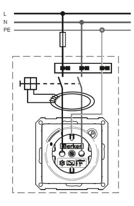
Figure 2: Connection with TN-S or TT network
