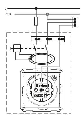
Figure 3: Connection with TN-C network
