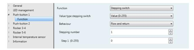
Figure 39: "Step switch" function"
