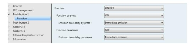
Figure 20: "Function by press/on release" parameters
