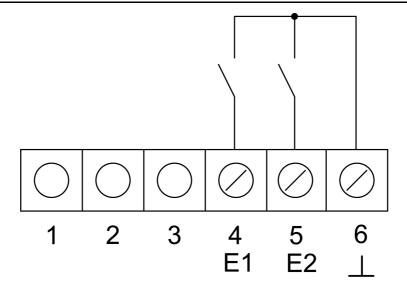
Figure 3: Connection of binary inputs
