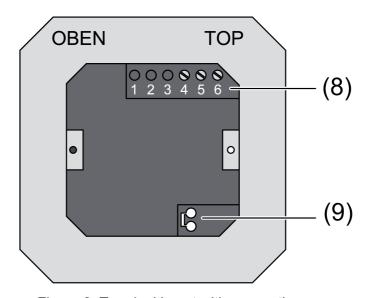
Figure 2: Terminal insert with connections
