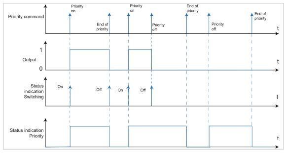
Figure 24: Signal-time diagram for Priority
