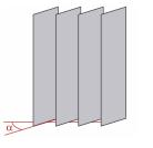
Slat angle in % – Fully closed slats arranged vertically  $\alpha \approx 0^{\circ}$
