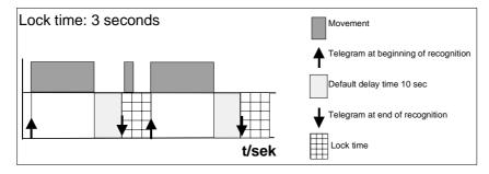
**Lock function:** The automatic function can be deactivated with the help of the lock function. The lock function can be triggered by any sensor of data type 1 bit, so that the corridor lighting can be switched on for a defined period independently of through traffic.
