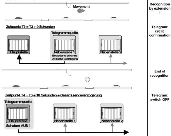
The heat source leaves the recognition range of extension 1. Extension 2 is installed in such a way that an enclosed recognition field is created and it can take over the function; it sends a telegram *Movement detected* to the master station.
