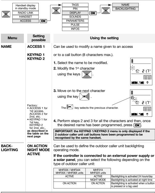
IMPORTANT: if a power cut occurs and the controller has battery back-up, backlighting is activated when a button is pressed or a badge used. If the controller is powered by a solar panel, ACTIVE must be selected. Backlighting will be enabled when a button is pressed or a tag used.
