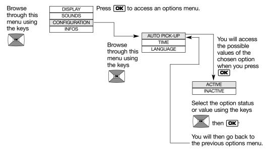
• Quickly press C to return to the previous display at any time.
