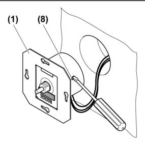
Figure 4: Adjusting basic brightness
