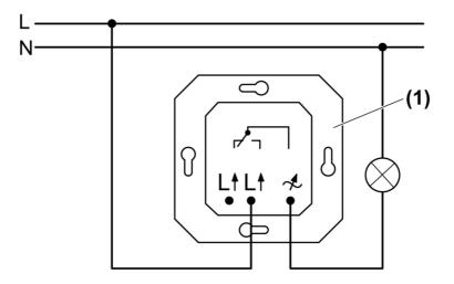
Figure 2: Connection diagram
