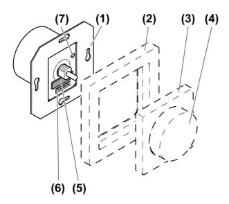
Figure 1: Device components
