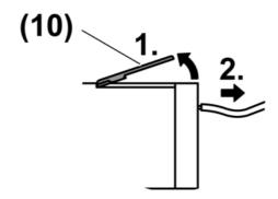
picture 4: Disconnecting the plug-in terminal
