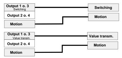
Switching the twilight level of the slaves on and off, where not parameterised to brightness-<u>in</u>dependent, is done by linking the output objects. An object value > 0 at the start of the detection causes the twilight level (brightness-<u>in</u>dependent) to be deactivated, and an object value = 0 after the additional transmission delay has elapsed causes the twilight level (brightness-dependent) to be activated.
