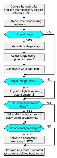
Once all devices (for instance masters and slaves in a project) have been configured and individually commissioned, it is recommended that a bus reset is performed, to create a defined base condition.
