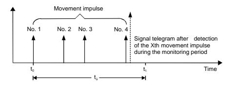
After detecting the 4th movement impulse (x = X) within the monitoring period t<sub>ü</sub>, a "report message after detecting the Xth movement impulse" is sent in accordance with the parameterisation.
