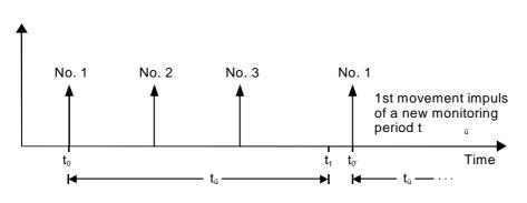
**<u>Case 2</u>**: x = 3 movement impulses are detected during the monitoring period  $t_{\hat{u}}$ .
