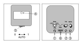
Changes the default "additional transmission delay" by ± 50 % (this potentiometer has no function in extension mode).
