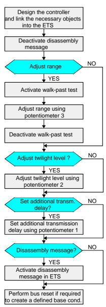
Once all devices (for instance masters and slaves in a project) have been configured and individually commissioned, it is recommended that a bus reset is performed, to create a defined base condition.
