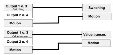
Switching the twilight level of the slaves on and off, where not parameterised to brightness-<u>in</u>dependent, is done by linking the output objects. An object value > 0 at the start of the detection causes the twilight level (brightness-<u>in</u>dependent) to be deactivated, and an object value = 0 after the additional transmission delay has elapsed causes the twilight level (brightness-dependent) to be activated.
