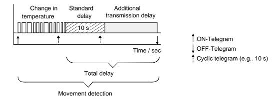
Messages can be sent for the start and the end of a movement detection. During a movement detection the controller is always in brightness-<u>independent mode</u>, i.e. it will trigger the start of the total delay count-down at each new movement detection, irrespective of the ambient brightness.
