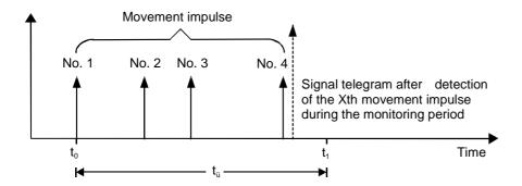
$\Rightarrow$  After detecting the 4th movement impulse (x = X) within the monitoring period  $t_{\bar{u}_i}$  a "report message after detecting the Xth movement impulse" is sent in accordance with the parameterisation.
