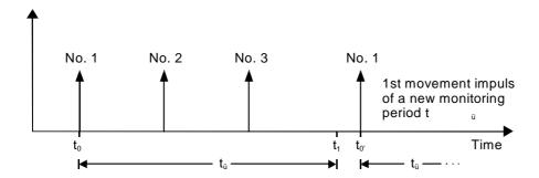
$\Rightarrow$  In the first monitoring period only 3 movement impulses (x < X) were detected. It follows that no report message is triggered. After  $t_{\ddot{u}}$  has elapsed the next movement impulse will be the first of a new monitoring period  $t_{\ddot{u}}$ .
