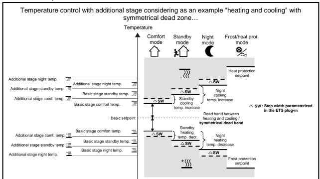
If enabled in the ETS, 6 temperature setpoints can be varied in "heating and cooling" control option. Depending on the temperature decrease, increase or dead zone parameterized in the ETS, all temperature setpoints are derived from the basic setpoint temperature.
