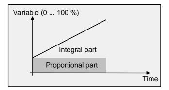
An additional PI controlled heating or cooling stage works exactly as the PI control of the basic stage. The difference is that the setpoint will shift by taking into account the parameterized stage offset.
