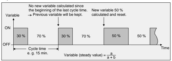
With an actuating variable of 0 % (continuously switched-off) or 100 % (continuously switched-on) an actuating variable telegram according to the actuating variable value ("0" or "1") is output after a cycle time has elapsed. With this type of control, the 'clipping' behaviour (cf. "continuous PI control") is active as well.
