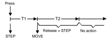
Pressing the key will transmit a step command and time T1 is started ("Time between short and long-time operation"). If the key is released within T1, no further telegram will be transmitted. This STEP serves the purpose of stopping a continuous move.
