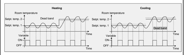
An additional 2-state control heating or cooling stage works in exactly the same way as the 2-state control of the basic stage. The difference is that the setpoint and the hysteresis values will shift by taking into account the parameterized stage offset.
