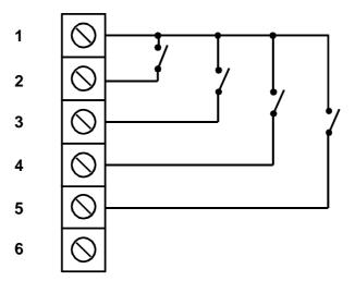
Example 2: implementation of 2 binary outputs,. 1 binary input, external temperature sensor recommended cable type:
