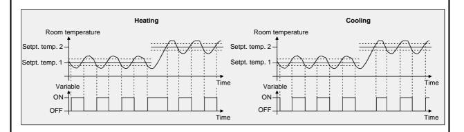
An additional 2-state control heating or cooling stage works in exactly the same way as the 2-state control of the basic stage. The difference is that the setpoint and the hysteresis values will shift by taking into account the parameterized stage offset.
