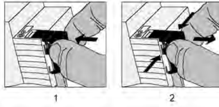
Figure 7: Installing / removing the protective cap for the bus connection
