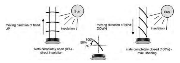
picture 31: Type 2 - slatted blinds with oblique and horizontal slat position
