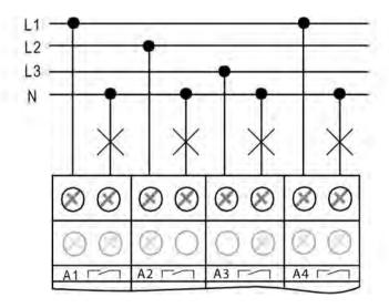
picture 4: Electrical connection for loads in switching operation
