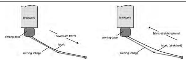
picture 50: Fabric-stretching in an awning
