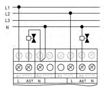
picture 5: Electrical connection for electrothermal valve drives
