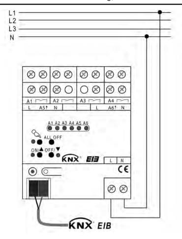
picture 2: Electrical connection of mains voltage
