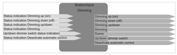
Figure 7: Input/output signals Dimming function
