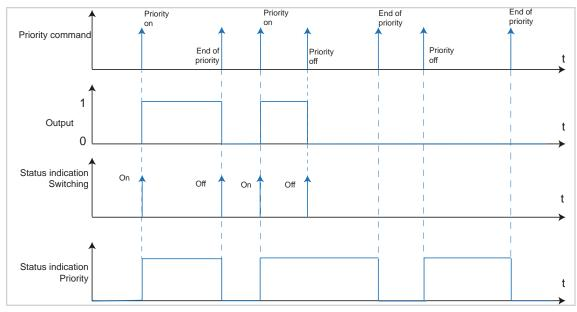
Figure 32: Signal-time diagram for Priority
