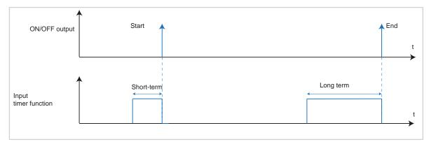
Figure 29: Signal-time diagram for timer
