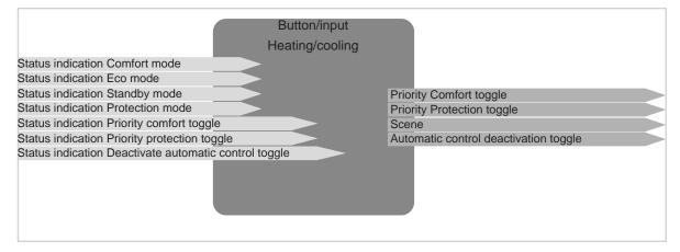
Figure 9: Input/output signals Heating/cooling function
