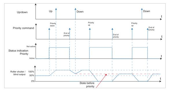
Figure 66: Signal-time diagram for **Priority roller shutter/blind**
