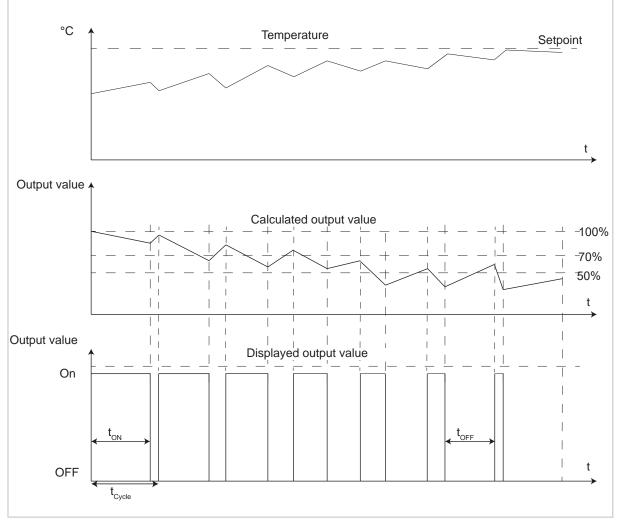
Figure 19: Switching PI-control (PWM)
