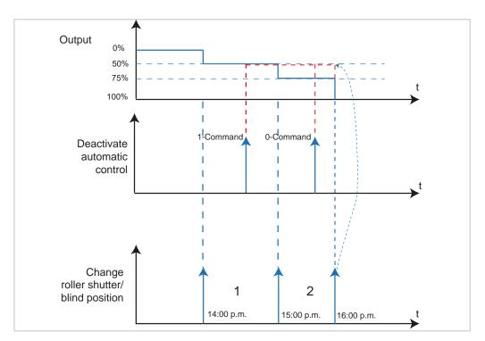
Figure 68: Signal-time diagram for Automatic control deactivation
