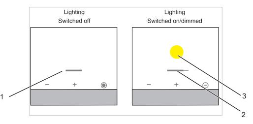
Figure 42: Display page Dimmer switch function
