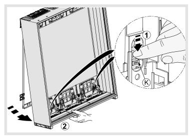
3. Removal quickset bracket (operating the K element)
