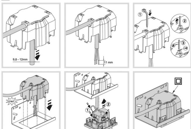
Mounting of the WH37961523Z cover for FLF sockets to ensure protection class II
