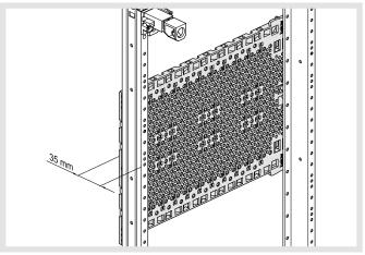
Installation of the UM00M0 plastic plate on the rear of the univers Z mounting rail
