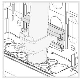
Fixing thick pipes to the plastic bottom part of the cabinet
