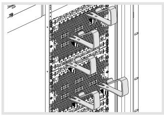
VZ02MM modem holder installed on the UM00M0 plate
