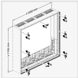
Finally, the brackets have to be fixed together with the frame using the PZ2 screws.
