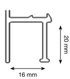
Integrated cable duct in the central area below the mounting rail
