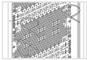
Cable ties installed on the UM00M0 plastic mounting plate
