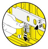
1. Removing the steel fixation frame
