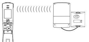
The Light button on the handset controls the lighting connected to the relay output receiver. The handset is considered as the transmitter while the output receiver acts as the receiver.
