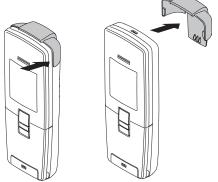
**3.** Replace the flat MTU01X battery with a new once.
