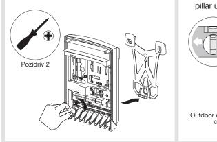
**2.** Following the installation rules below, mark 3 fixing points and drill a hole in the pillar using a Ø 6 mm drill bit.
