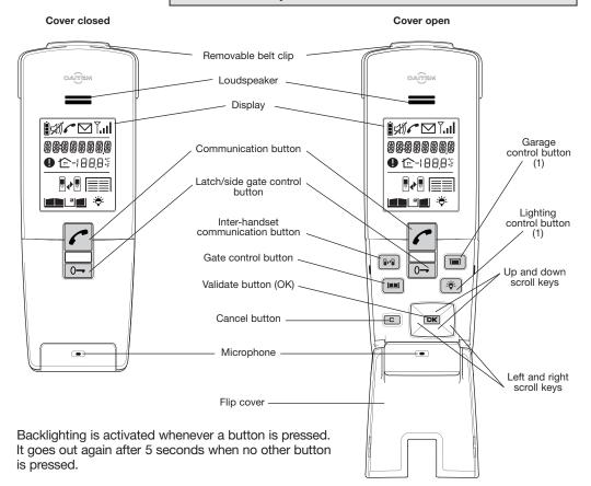
(1) These functions require a relay output receiver to be installed.
