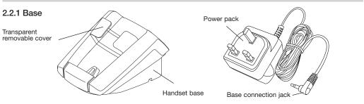
IMPORTANT: when installing the system, the handset(s) must be charged on their base before they can be used.
