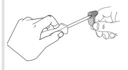
2. Cut the cables to the necessary length and then thread them through the grommets. Expose the end of the wires over a length of approximately 1 cm.
