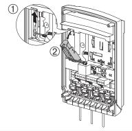
4. Remove the flat battery from its box.
