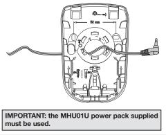
**5.** Connect the jack to the base making sure that the cable is positioned in the designated slot.
