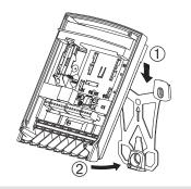
5. Lock the base in place using the locking screw.
