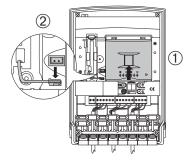
3. Remove the battery enclosure.
