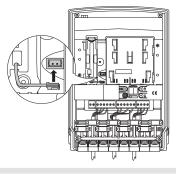
8. Connect a new MPU01X battery.
