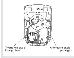
**11.** Feed the power cable through one of the guides on the back of the base.
