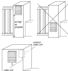
Do not place the products near metal surfaces (screens, fences, gates, etc.) or sources of electromagnetic disturbance:
