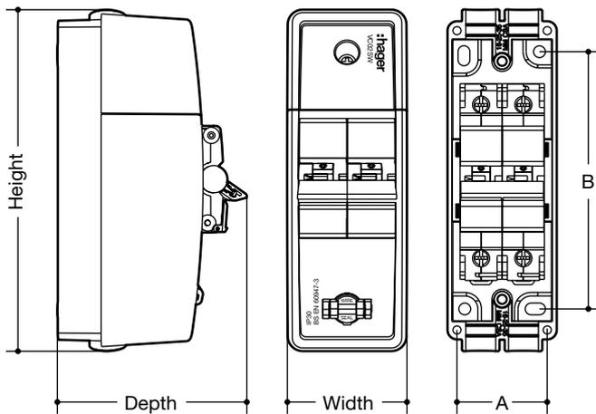
VC02SW is an Enclosed Switch Disconnecter suitable for Meter Box Applications where an isolating switch between the electricity meter and consumer unit is required.
