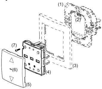
Figure 1: Design and layout of the device
