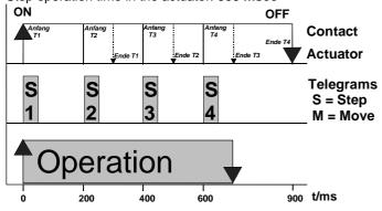
Activation for approx. 700 msec. Four step commands are sent. After the 4th step command (t = 600 msec) the total short-operations time runs through in the actuator, so that the actuator releases the drive after about 900 msec.
