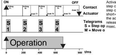
Activation for approx. 700 msec. Four step commands are sent. After the 4th step command (t = 600 msec) the total short-operations time runs through in the actuator, so that the actuator releases the drive after about 900
