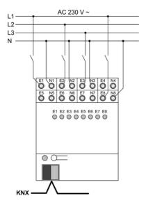
picture 3: Connection example for 230 V binary inputs
