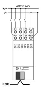
picture 4: Connection example for 24 V binary input
