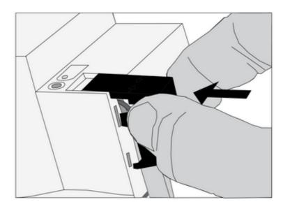
picture 6: Installing the cover
