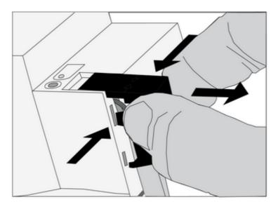
picture 7: Removing the cover
