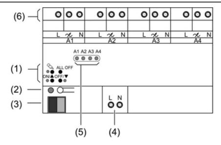
Figure 2: View of dimmer actuator 4-gang
