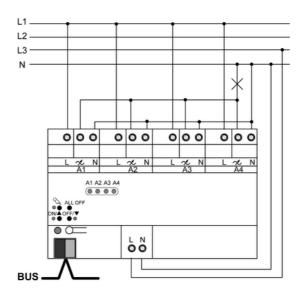
Figure 5: Parallel switching of dimmer outputs – connection example
