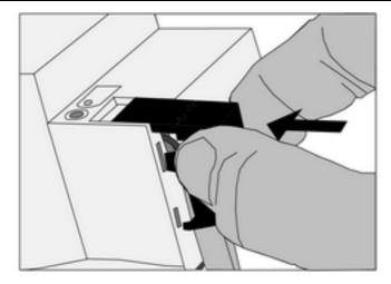
Figure 7: Installing the cover
