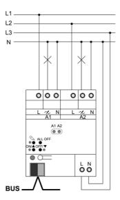
Figure 4: Dimmer actuator - Connection example
