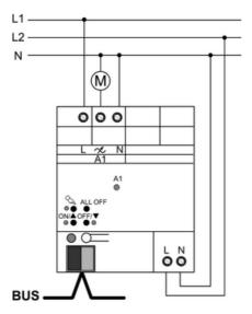
Figure 6: Dimmer actuator 1-gang – connection for speed controller operation
