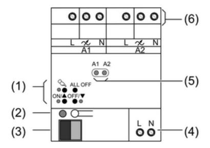
Figure 1: View of dimmer actuator 2-gang
