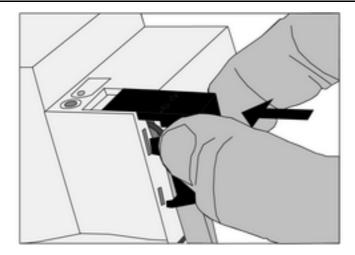
Figure 3: Installing the cover
