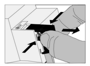
Figure 4: Removing the cover
