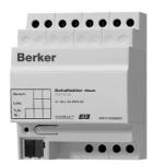
The switch actuator receives telegrams via the EIB and switches groups of electrical equipment with its six potential-free independent relay contacts. Various external conductors can be connected.
