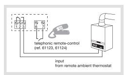
Connection of the thermostat to the thermostat input of a reversible or irreversible heat pump
