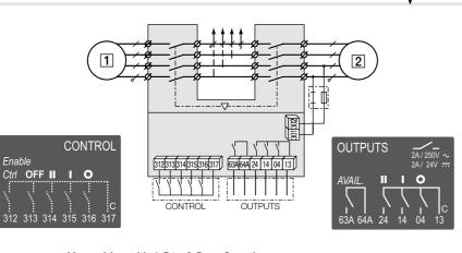
Use cables with 1,5 to 2,5 mm<sup>2</sup> section. Screw M3 - Tightening torque: min.: 0.5 Nm - max.: 0.6 Nm
