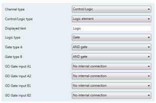
Fig. 24: Logic element
