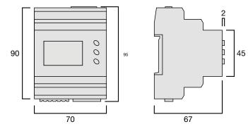
Please allow space above and below the meter for cable connections.
