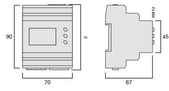
Please allow space above and below the meter for cable connections.
