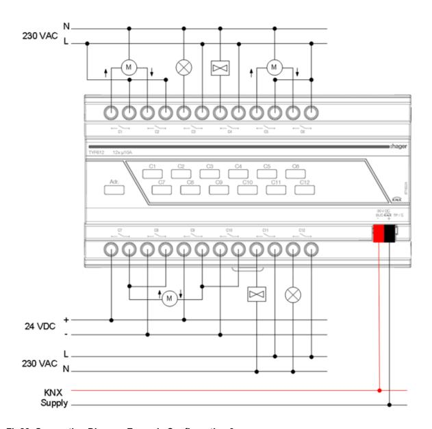
Fig23. Connection Diagram Example Configuration 3
