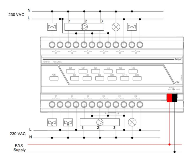
Fig22. Connection diagram example Configuration 2
