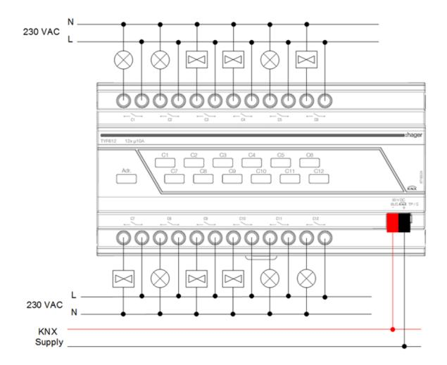
Fig21. Connection Diagram Example Configuration 1
