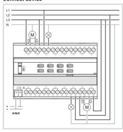
Fig 2: Device connection
