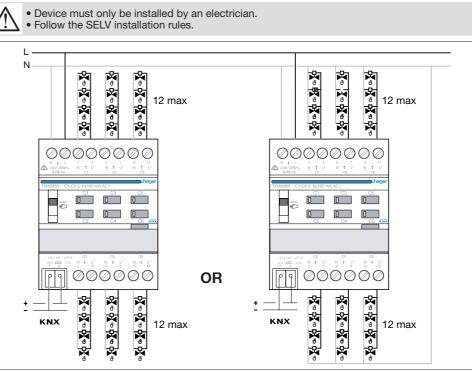
Image 3: valves equipped with thermal actuators with 230 V ~ power supply
