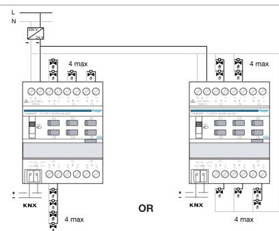
Image 4: valves equipped with thermal actuators with 24 V ~ power supply
