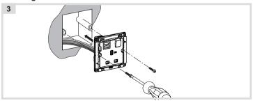
After wiring, fix the device with the two screws attached into the wall box (3).
